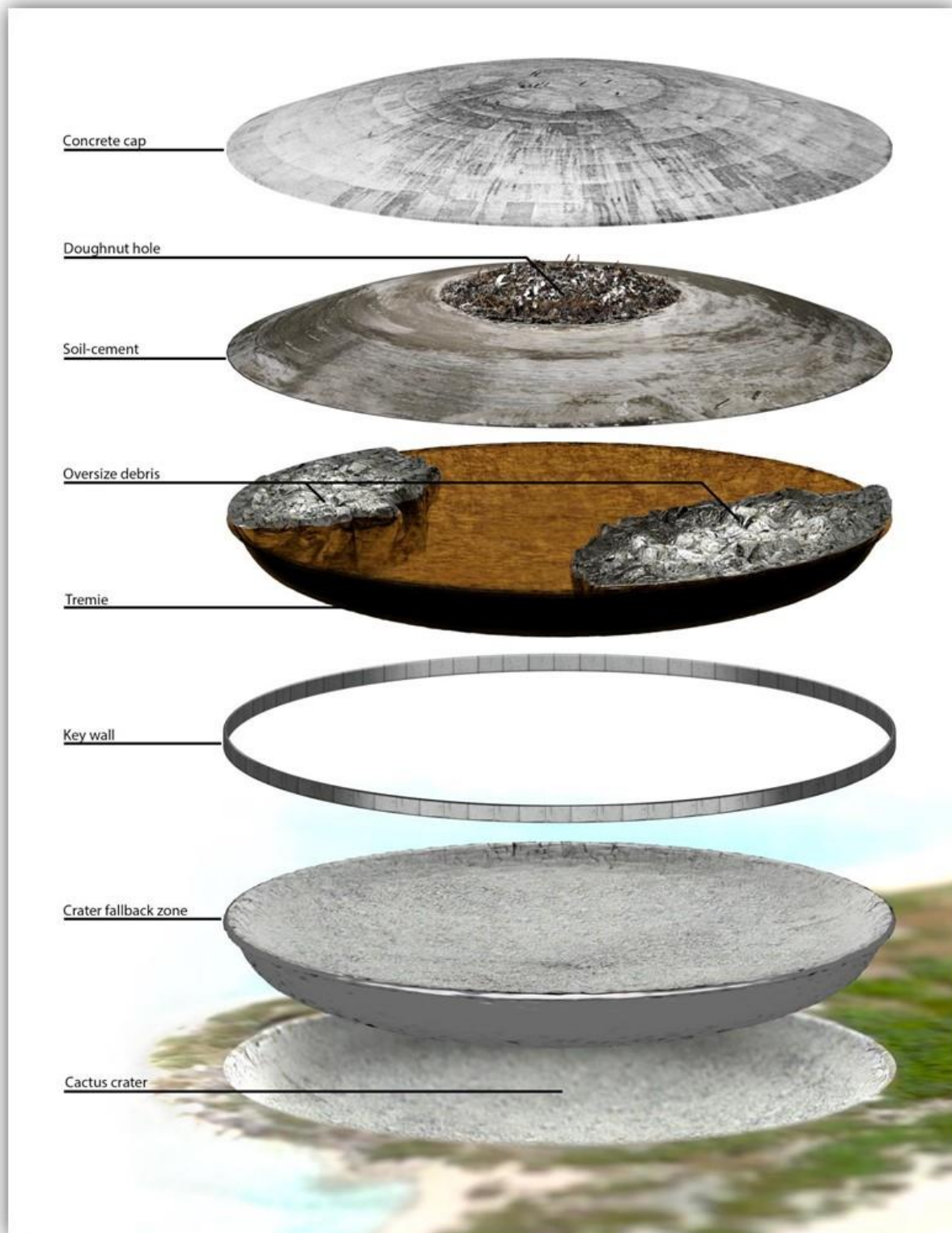
Design elements of the Cactus Crater containment structure
