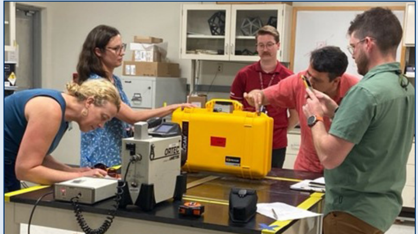
PROACTIVE team members perform a gamma-ray measurement to determine the absence of special nuclear material in a simulated weapons part, as part of a larger verification system exercise at ORNL in August 2023. During the experiment, a building was configured as a mock materials storage facility and outfitted with a variety of sensors including door switches, motion detectors, spectroscopic portal monitors, and cameras. The intent of the experiment was to test and validate a framework for collecting data from a variety of different sensor types, then confirming, storing, and analyzing that data to inform a picture of the facility and identify potential vulnerabilities in the verification process.
